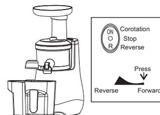
After the squeezing process is completed, please press the stop switch, and pull out the power plug.
