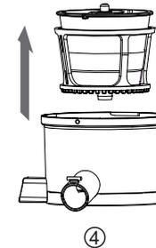
5. Respectively disassemble the spiral propeller, squeezing barrel and washing rack.
